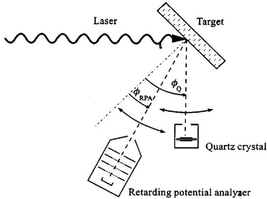
FIG. 1. Schematic diagram of the experimental setup. The laser pulse is incident at a fixed angle of  $45^\circ$ . Particle analysis is in the plane of incidence by a combination of a retarding potential analyzer and a quartz crystal.
